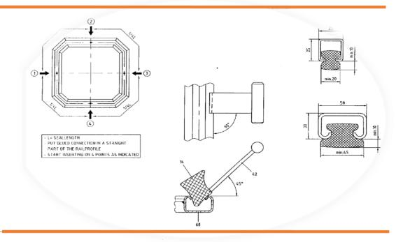
Badly Worn or damaged seals should be re-placed prior to use. New seals can be inserted into seal profile using insert bar at an angle of 45 Deg, see diagram above.
